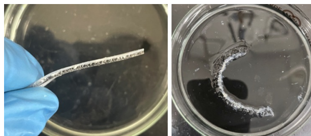
Figure 6. Bending actuation in THF by PDMS-acrylate bilayer sample. Left is before and right is after putting in THF.
