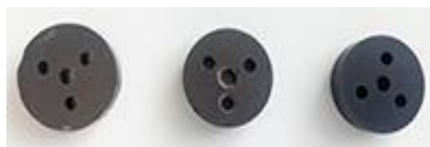
Fig. 5. Top view of the drilled bulk \text{MgB}_2
