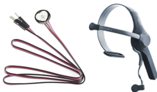
Fig.3. Biological sensors used in the experiment: (a) pulse sensor (b) brainwave sensor
