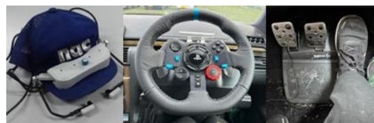
Fig.4 Nac eyemark recorder and Steering controller (logicool: LPRC-15000d)
