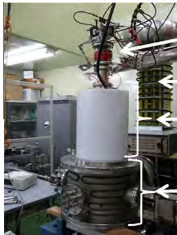
Fig. 2. Photograph of the compact microbeam system with a high-voltage power supply (300 keV) and a vacuum chamber placed next to it. The system is placed in air in a typical size laboratory.
