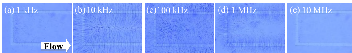
Figure 3. Dielectrophoretic trapping of Ag nanowires at various frequencies.
