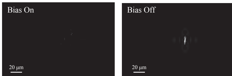
Fig. 6. Preliminary results for interferometer function on the PDMS MZ waveguide with a titanium filament. Light transmission was disrupted by applying voltage to the filament. Heat transfer to the sample was not measured, but light transmission was recovered by removing the voltage from the filament.
