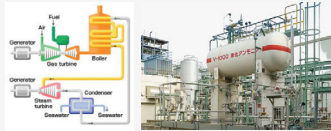
Combined cycle power generation
