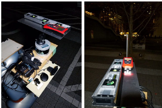
Measuring the distance by using LKT-F05 between vehicle and landmark
