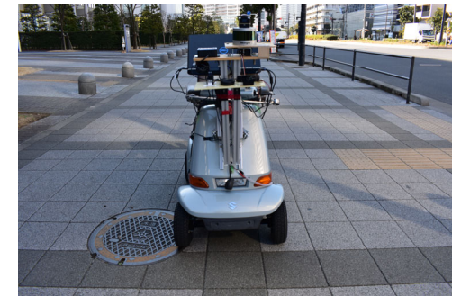
LiDAR sensor attached to the senior car
